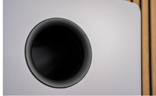
The Move has a bass reflex tuning in favour of strengthening the low frequencies. The port rounded at the mouth, completely burr-free in the tube and thus overall flow-optimised is positioned on the back of the monitor.
