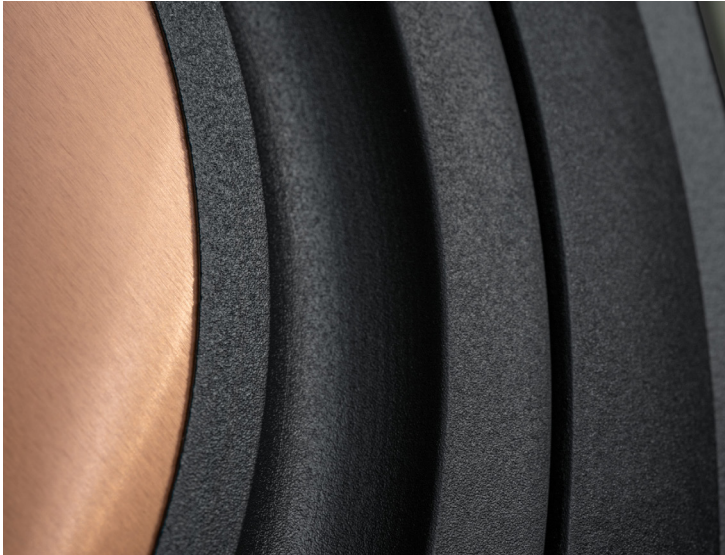
The sophisticated enclosure is also the only guide of the diaphragm: The full-range chassis operates without a centring spider. That is why this mono suspension is realised in a special inverse shape and with four synthetic materials.
