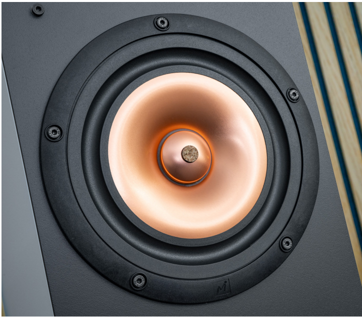
The full-range speaker handles sound conversion from 40 to 10 kilohertz. This is how the Move acts as a point sound source.
