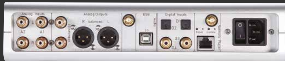
◀ Musicbook combines an amazing variety of gold-plated connectors on its rear panel
