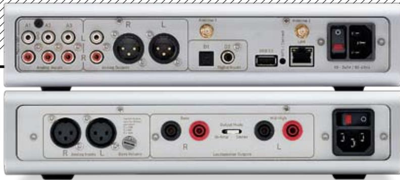
**ABOVE:** The pre/DAC [top] includes USB-A, optical and coaxial digital and network ins plus WLAN/BT antennae alongside three line ins and balanced/single-ended pre outputs. The 1000 Power [bottom] offers balanced inputs only and 4mm speaker output sockets. In 'Bi-Amp' mode the gain/volume of the R channel is variable
