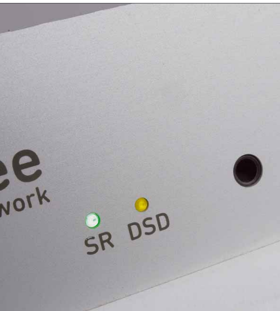
The LEDs provide information about the sampling rate used and the DSD mode
