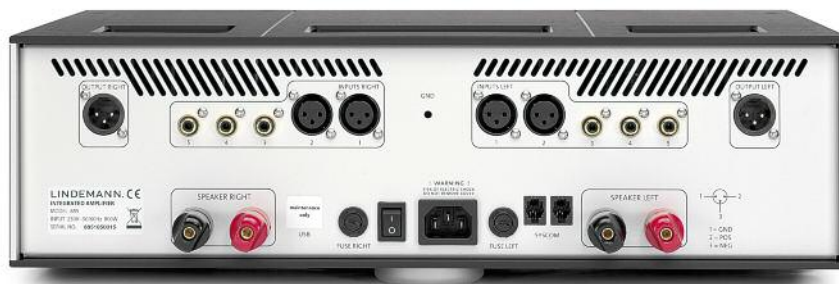
The connector panel reveals the double-mono configuration
