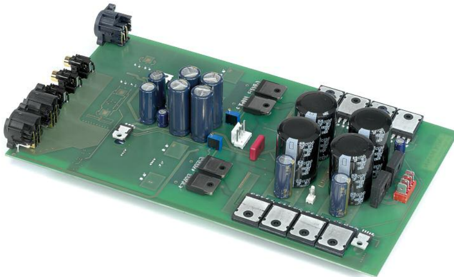
The upper side of the main circuit board also houses the end transistors
